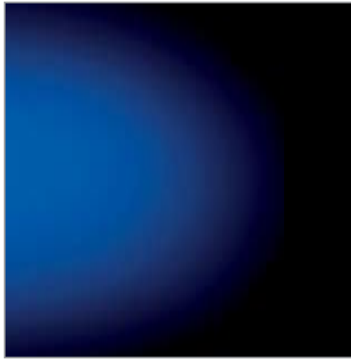
Projection from 3 meters with beam shaper system.
